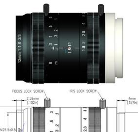
M25.5x0.5 S0mm [1.181in] MAXIMUM OUTER DIAMETER 50 4mm [1.984in] 50 4mm [1.984in]
